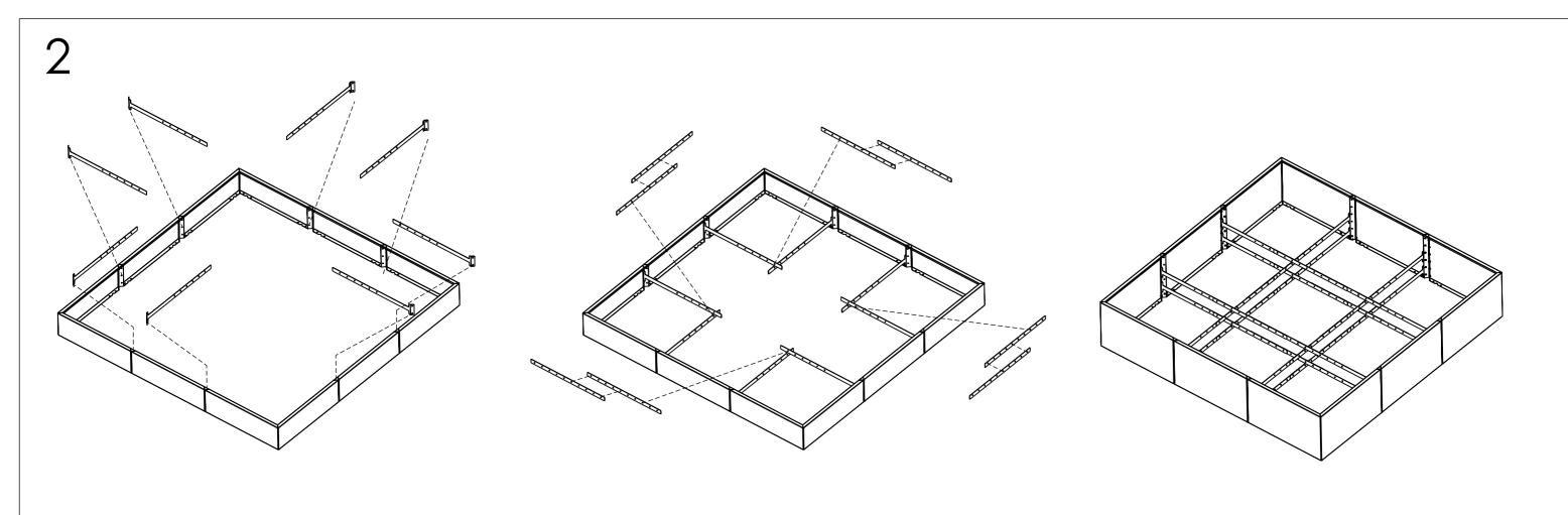
Models from height 500mm 2 connecting struts one above the other
